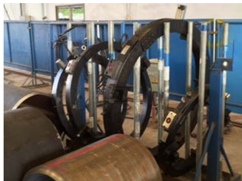
Piping Cutting/ Beveling MC : 12"~46" (5 sets)
